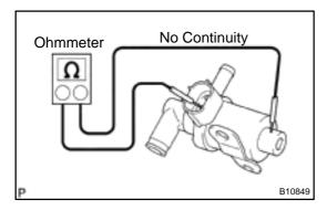
(b) Inspect the VSV for ground. Using an ohmmeter, check that there is no continuity between each terminal and the body.
